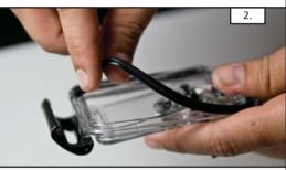
3. To install a new or clean T-Seal, start at any corner, push the T-Seal into the corner and run your finger along the T-Seal pushing it into the Case Contact Surface.
